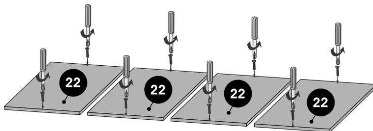
UTILIZAR TORNILLO AUTOPERFORANTE LARGO
